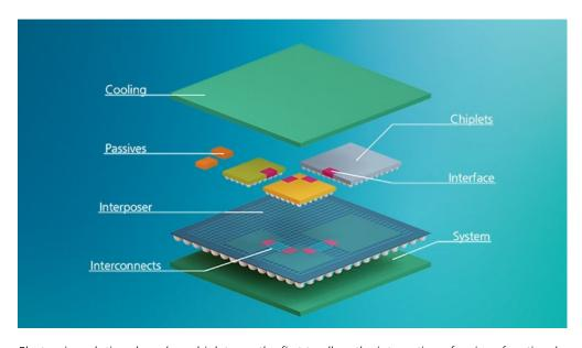
Electronics solutions based on chiplets are the first to allow the integration of various functional units in different technologies on a substrate or into a 3D chip structure, © Fraunhofer IIS/EAS
